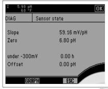
Sensor monitor, numerical display (example)
