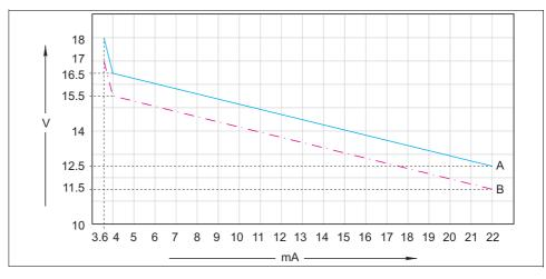
Minimum supply voltage at the transmitter depending on the output current
