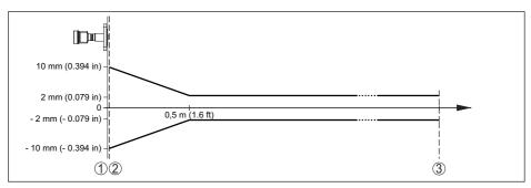
Fig. 38: Deviation under reference conditions
