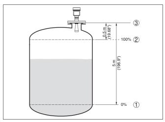
Fig. 32: Parameterisation example, Min./max. adjustment
