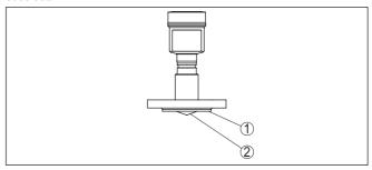
Fig. 8: VEGAPULS 63 with flange and encapsulated antenna system
