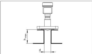
Fig. 7: Deviating socket dimensions
