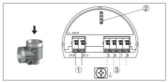
Fig. 22: Electronics compartment - Ex-d-ia double chamber housing
