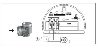
Fig. 21: Connection compartment - Radio module PLICSMOBILE 81
