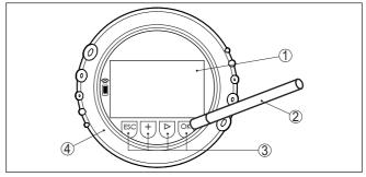
Fig. 31: Display and adjustment elements - with adjustment via magnetic pen
