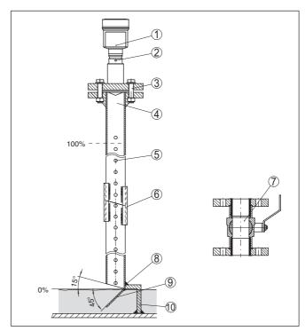
Fig. 14: Configuration surge pipe VEGAPULS 63
