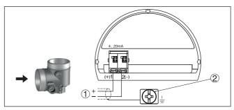
Fig. 23: Connection compartment - Ex-d-ia double chamber housing
