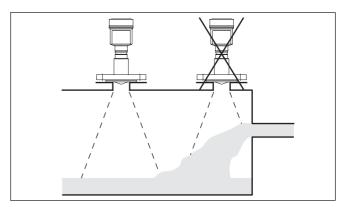
Fig. 6: Mounting of the radar sensor with inflowing medium
