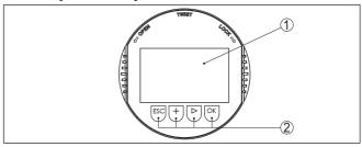
Fig. 30: Display and adjustment elements
