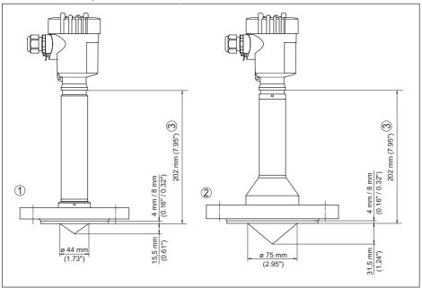
Fig. 45: VEGAPULS 63, flange version, low temperature
