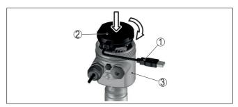
Fig. 33: Connection of the PC directly to the sensor via the interface adapter
