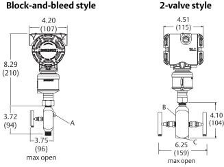
A. Bleed screw (unspecified dimension) - not  $\,$  C.  $^{1}/2-14$  NPT female NPT process connection (code BA) designed for accessory attachments.
