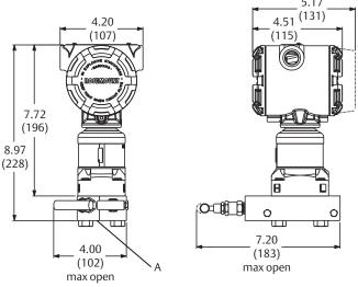
A.  $^{1}/_{2}$ –14 NPT on manifold for process connection,  $^{1}/_{4}$ –18 NPT for test/vent connection Dimensions are in inches (millimeters).
