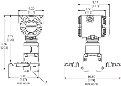
A.  $^{1}/_{2}$ -14 NPT on manifold for process connections,  $2^{1}/_{8}$ -in. center-to-center,  $^{1}/_{4}$ -18 NPT for test/vent connection Dimensions are in inches (millimeters).
