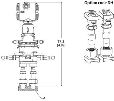
A. Cross section image is shown for dimensioning purposes only; it is not part of the transmitter assembly Dimensions are in inches (millimeters).
