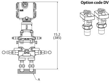
A. Cross section image is shown for dimensioning purposes only; it is not part of the transmitter assembly Dimensions are in inches (millimeters).
