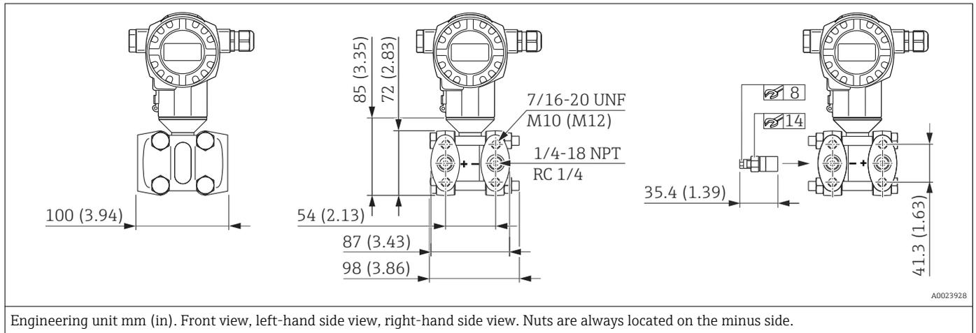
Engineering unit mm (in). Front view, left-hand side view, right-hand side view. Nuts are always located on the minus side.
