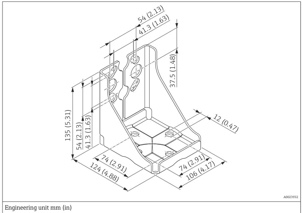
Bracket for wall and pipe mounting including retaining bracket for pipe mounting and two nuts
