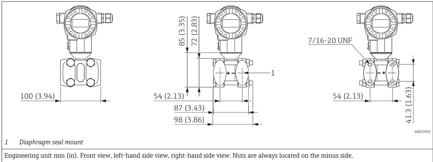
**Process connections FMD78 with diaphragm seal**
