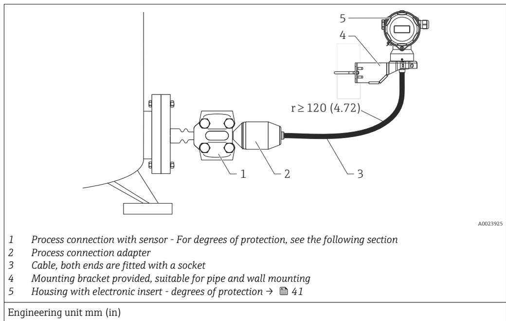
Degree of protection for the process connection and sensor with the use of
